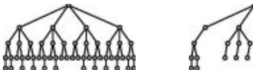
Figure 8.2: Left: The game tree of a 2 \times 2 Hex game in an arbitrary ordering. The minimax algorithm must visit all 52 nodes before determining the value of the game and the best move. Right: By this ordering of moves, the alpha-beta-algorithm succeeds in truncating the game tree of 2 \times 2 Hex to 13 nodes in determining optimum result for both players—not when devising a winning strategy.
